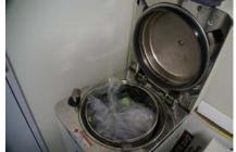
Operate the autoclave using wet heat at 120°C or higher for 20 minutes or more. Ensure sufficient space between containers to maximize the effect of wet heat on microbes.
