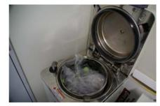
Operate the autoclave using wet heat at 120°C or higher for 20 minutes or more. Ensure sufficient space between containers to maximize the effect of wet heat on microbes.
